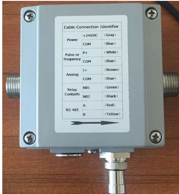
Fig. 3 Cable Connection Identifier
