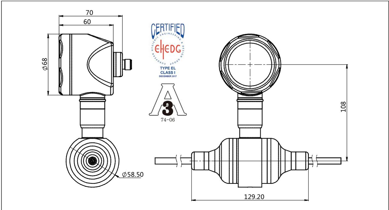
Drawing and dimension with display (C) / without display (A) horizontal installation (F2) (unit: mm)
