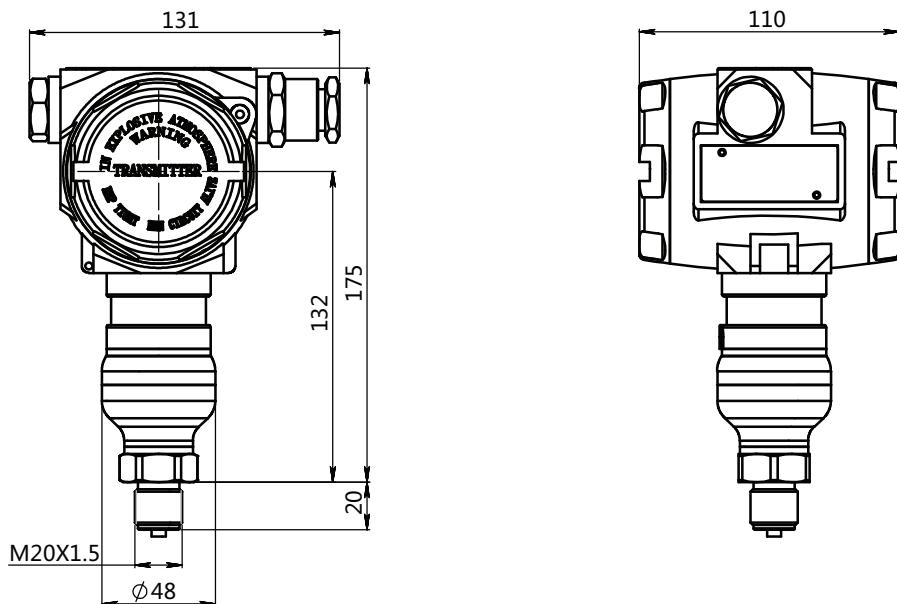
Drawing and dimension of DMP305X-TST-H without display(A) ( unit: mm)
