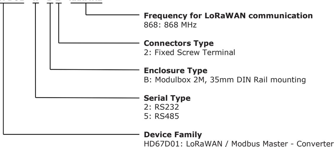
Order Code: **HD67D01-2-B2-868MHz** - LoRaWAN / Modbus Master – Converter (RS232)
