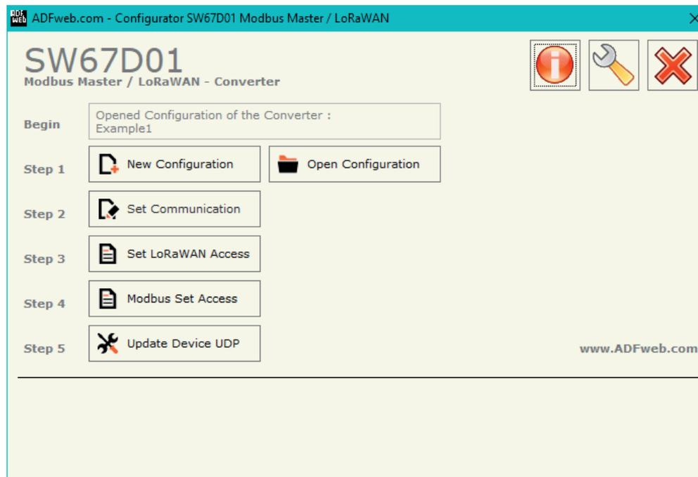
Figure 2: Main window for SW67D01
